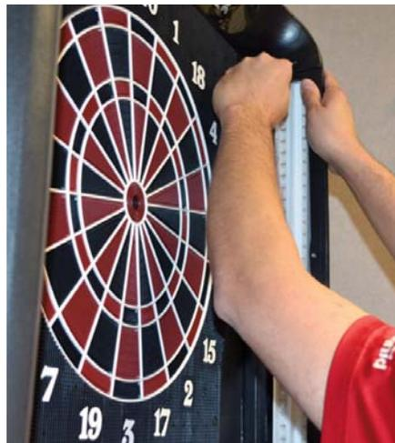
7. Slide the Target Light Fixture out of the opening.
