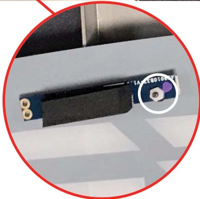
4. Remove the Camera from the Marquee using a  $\frac{3}{16}$ " nut driver.
