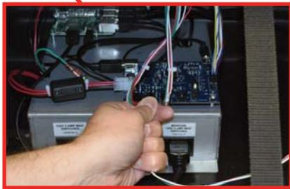
6. Unplug the Camera from the Control Board. It will be easier to remove and replace the marquee.
